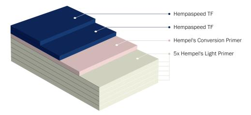
For a full season protection, the substrate needs to be sealed with Hempel's Light Primer (300µm dft) before applying Hempel's Conversion Primer and 2 coats of Hempaspeed TF. Follow stated overcoating intervals between the primer and product to ensure intercoat adhesion.
